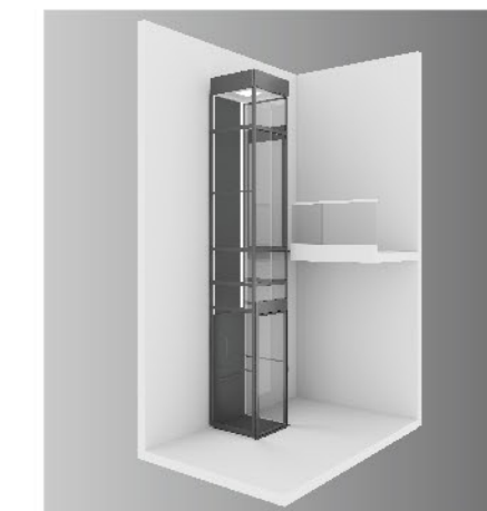
顶层复式公寓小空间无底坑方案 Scheme of small space bottomless pit in penthouse apartment
